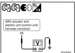
Turn ignition switch OFF and check continuity between ABS actuator and electric unit (control unit) harness connector E30 terminals 1, 4 and ground.
