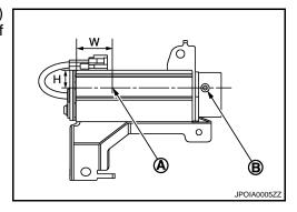
• To identify the center of laser beam axis (A) easily, prepare a piece of paper (B) cut to the size of 38 mm (1.5 in) (W)  $\times$  22mm (0.87 in) (H) and attach it on the upper left point of the ICC sensor integrated unit (1).
