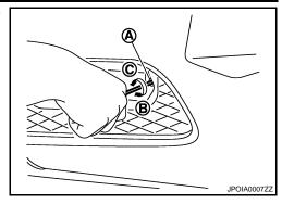
5. When "U/D CORRECT" value indicates ±4, confirm that the margin of value remains within ±4 at least for 2 seconds with no equipment or hand touching the ICC sensor integrated unit. When "COMPLETED THE VERTICAL AIMING OF LASER BEAM" appears on screen, touch "END". CAUTION:
