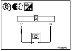
Check continuity between ECM harness connector and ground. VQ35HR
